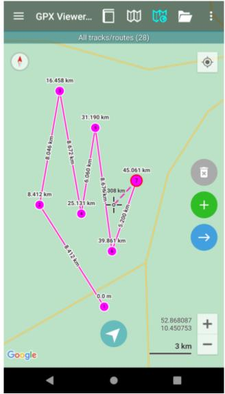
The numbers by the point mark the distance from the initial point based on the measurement line. The number on the line marks distance between two points connected by it.
