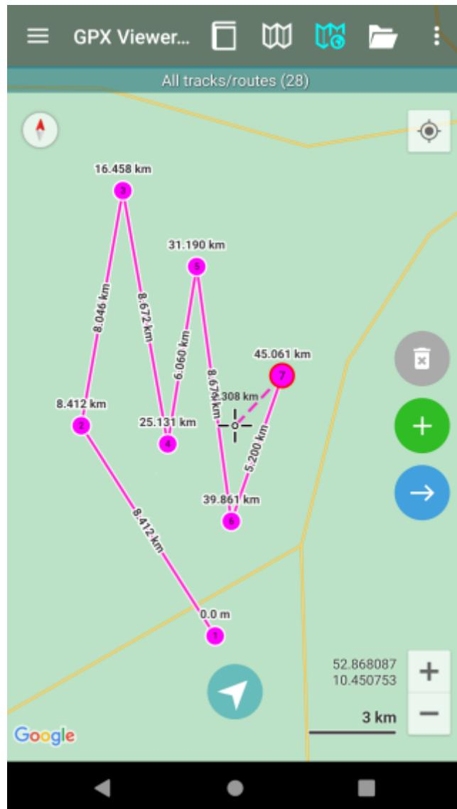
The numbers by the point mark the distance from the initial point based on the measurement line. The number on the line marks distance between two points connected by it. The distance measurement can not be used in the same time as track recording.
