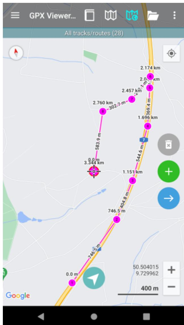
The numbers by the point mark the distance from the initial point based on the measurement line. The number on the line marks the distance between two points connected by it. The distance measurement can not be used at the same time as track recording.
