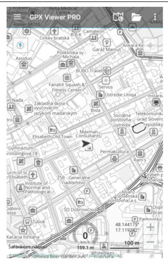
• Detail level - users can choose how many details the map will display; 0 - no details, no contours of objects; 11 - all of the details are displayed on the map. Only available for Refill, Tron, and Walkabout style. (On the pictures displayed levels 2,5,11.)
