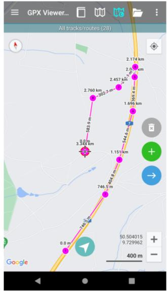
The numbers by the point mark the distance from the initial point based on the measurement line. The number on the line marks distance between two points connected by it. The distance measurement can not be used in the same time as track recording. update: 2022/09/30 13:12
